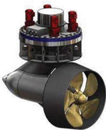
Figure 31. Azimuthing propulsor with nozzled propeller. [Image courtesy of Marine Propulsion Solutions.]
