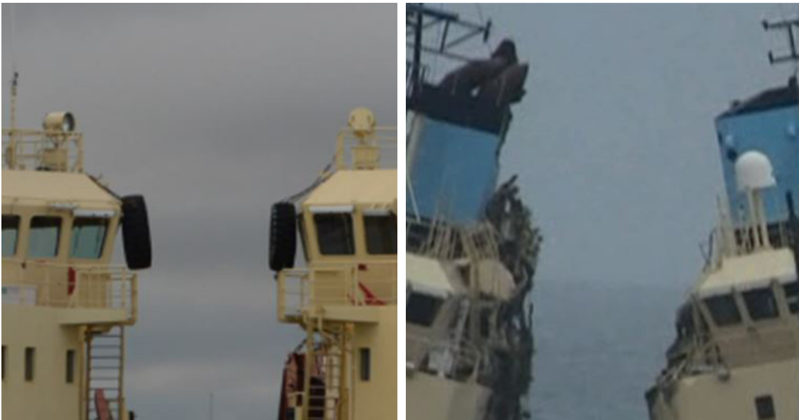
Figure 20: Left: Tyre fenders on bridge wings Right: Bridge wings after impact. Source: Maersk Supply Service
