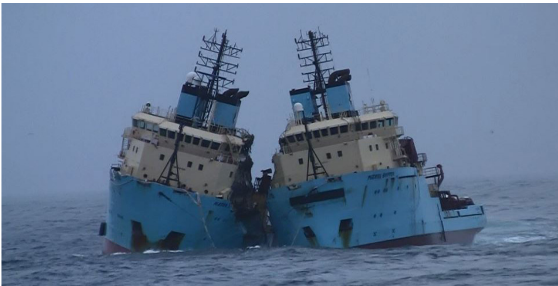
Figure 25: MÆRSK SHIPPER and SEARCHER with structural damage. Source: Maersk Supply Service
