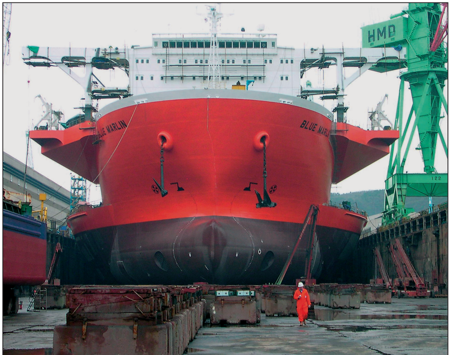
Blue Marlin in drydock at Hyundai Mipo Dockyard, where the enormous extra width of the vessel (exceptionally wide at 63m, compared with 42m previously) only just fitted into the dock.
