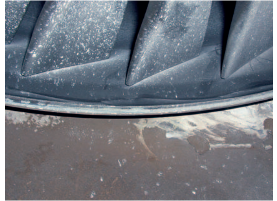
Worn turbine blade tips and turbine diffuser.
