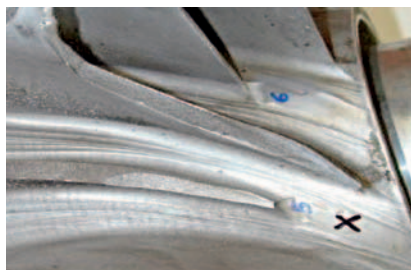
Damaged inducer wheel.
