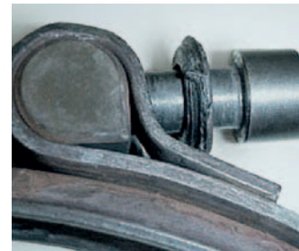
Deformed or wrong washer.
