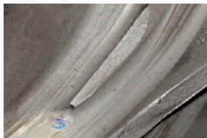
Close-up of a broken splitter blade.
