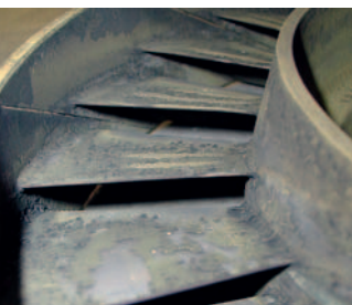
Components still very clean: cleaning intervals could be longer.
