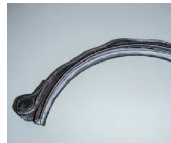
Cover tape severely deformed.
