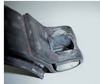
Severe wear at screw-head.
