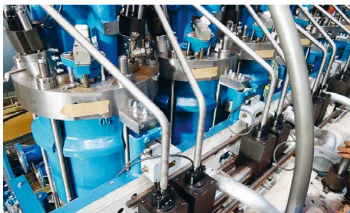
Common-rail system on Wärtsilä X35 engine.
