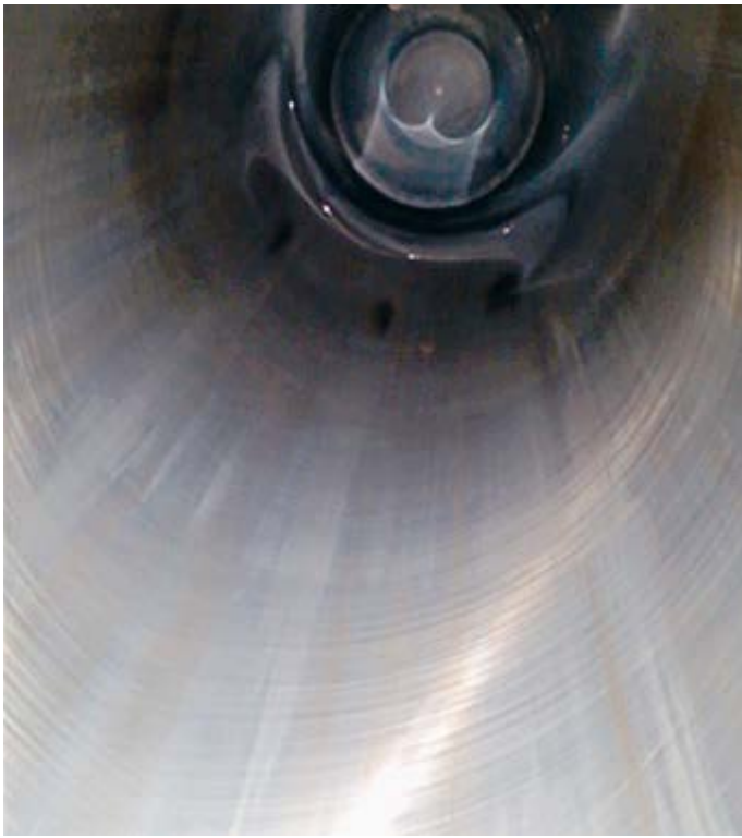
W-X82 cylinder liner after 1850 running hours. Honing marks well visible on the bottom part.
