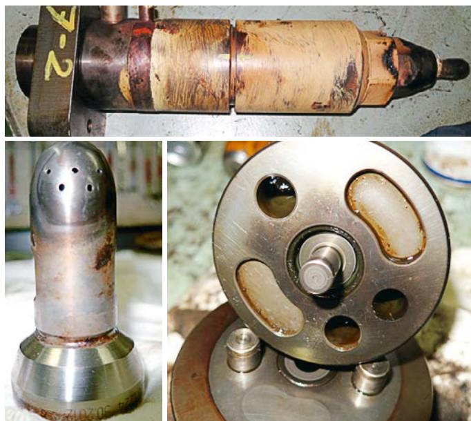
Different components of FAST injector inspected after 12'600 rhs.
