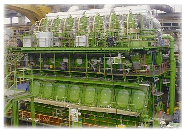
Figure 5 - The first MAN B+W 8-cylinder K98 engine, on test at Hyundai
