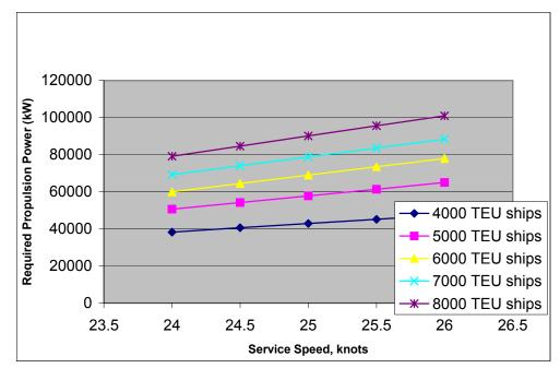
Figure 1 - Container ship Size vs Speed & Power
