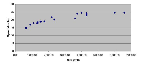
Figure 3 - Size vs Speed for current Maersk-SeaLand fleet
