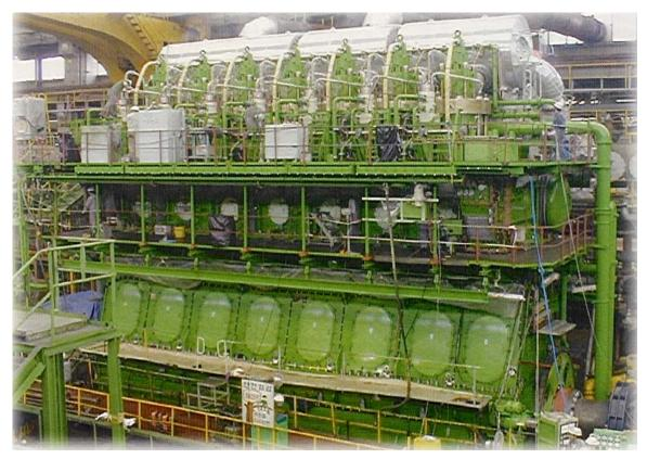
Figure 1 - The first MAN B+W 8-cylinder K98 engine, on test at Hyundai
