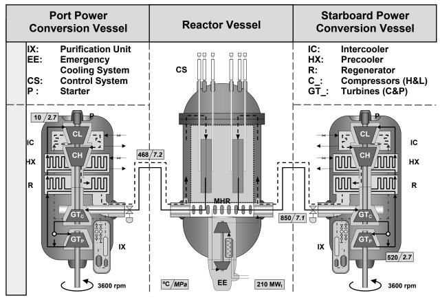
Figure 2 - Helium Flow Circuit in a GT-MHR Propulsion Module
