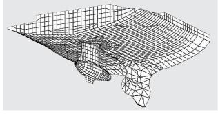
Fig. 11 FEM model of pod support structure
