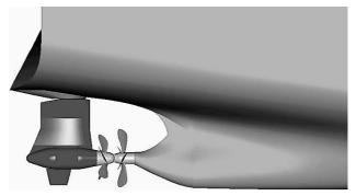
Fig. 3 CRP POD propulsion system
