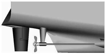
Fig. 2 Conventional twin shafts ship (shaft bracket system)
