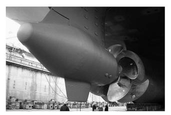
Fig. 1 CRP POD propulsion system
