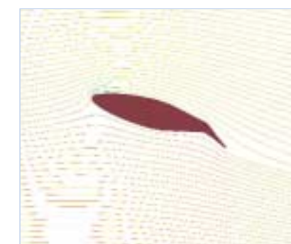
The illustration visualises the hydrodynamics for flap rudders.
