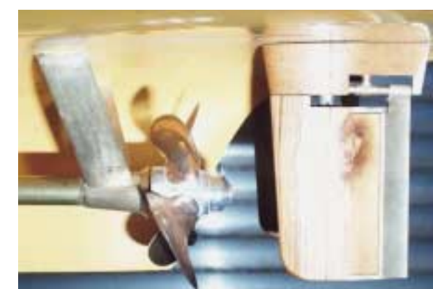
Scaled down models are tested to ensure optimum integration between the rudder, propeller and hull (HSVA).
