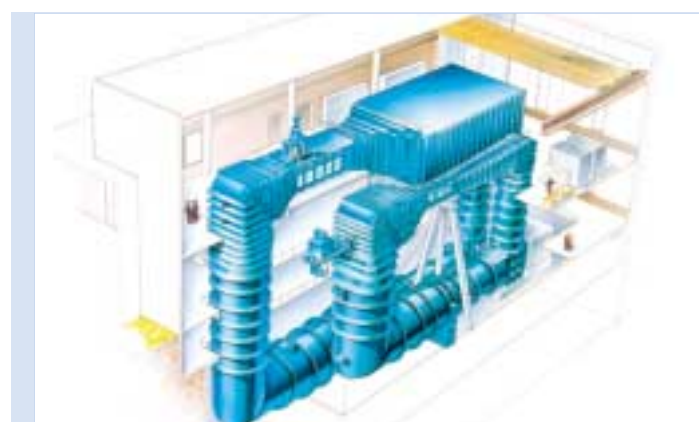
The hydrodynamic test centre in Sweden is equipped with two cavitation tunnels, enabling us to optimise manoeuvring equipment on any type of vessel.
