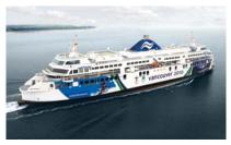
*RoPax Ferry "Coastal Renaissance" with double end propulsion drives 2 x 11 MW*
