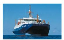
Research & trial vessel "Planet" with permanent excited propulsion motors 4 x 1040 kW and permanent excited main alternators
