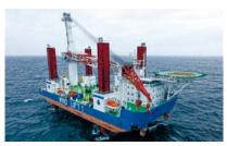
*Jack-up vessel "Windlift I" with PWM Active Front End (AFE) propulsion drives 4 x 1100 kW*
