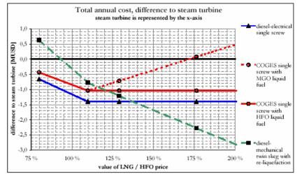
Figure 9 Total annual cost, versus the ratio of LNG value and HFO price, presented as difference to the steam-mechanical machinery
