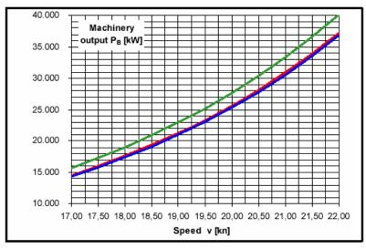
**Figure 3: Predicted Brake Power Requirements**
