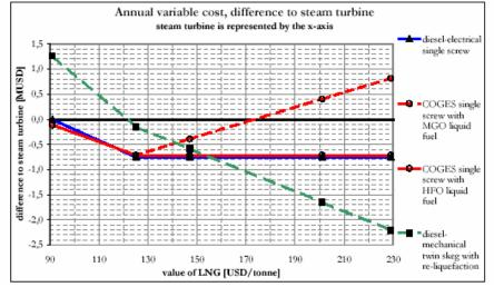
Figure 8 Recurring annual variable cost, versus the value of LNG, presented as difference to the steam-mechanical machinery
