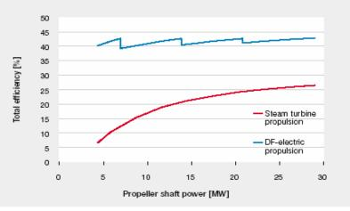
Fig. 2 Efficiency comparison between DF-electric and steam turbine propulsion for the case quoted in this article. The difference in needed power is merely due to different efficiency losses between the propeller and the engine or turbine. Since the diesel-electric version is producing electrical power, the loss of efficiency is greater than for the mechanically driven propeller.
