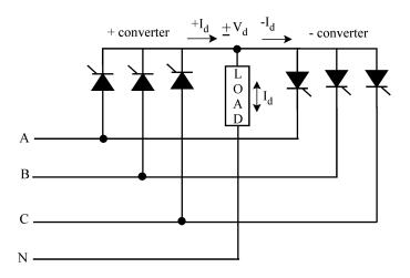
Fig. 4 3¢-1¢ half-wave cycloconverter
