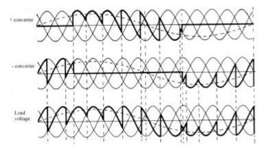
Fig. 10 Blocking mode operation waveforms
