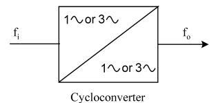
Fig.1 Block diagram of a cycloconverter
