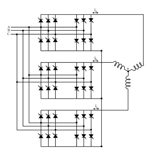
Fig. 8 30-30 bridge cycloconverter
