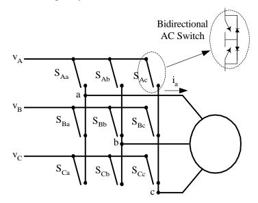
Fig. 12 Matrix converter
