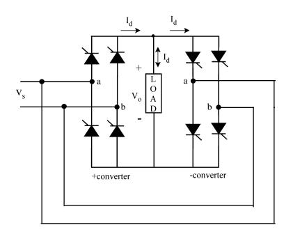
Fig. 2 Single-phase to single-phase cycloconverter
