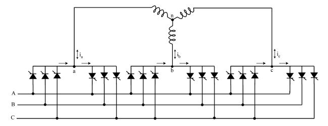
Fig. 7 30-30 half-wave cycloconverter
