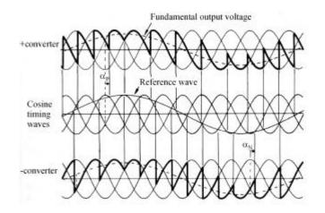
Fig. 6 30-10 half-wave cycloconverter waveforms
