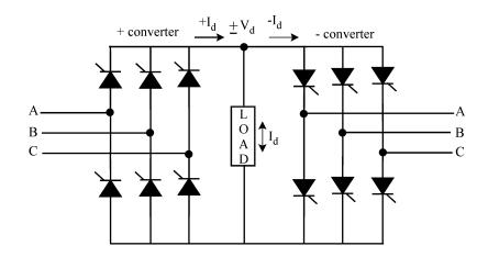
**Fig. 5** 3 $\phi$ -1 $\phi$  bridge cycloconverter
