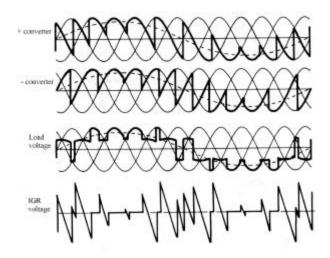
Fig. 11 Circulating mode operation waveforms
