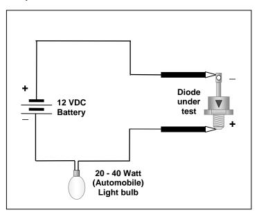
A good diode will light the bulb in only one direction. It should not light when test leads are reversed on the diode pin and base.
