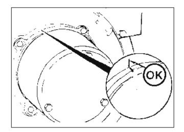
The radial position of the PMG Stator was important for adjustment of the AVR response and regulation.
