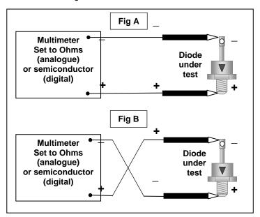
An electronic digital instrument will read true electron flow, hence the resistance polarity readings will be reverse to conventional current flow, i.e. forward and reverse readings will be reversed. A Digital Multimeter usually has a semiconductor test scale on the selector switch, marked as shown :-
