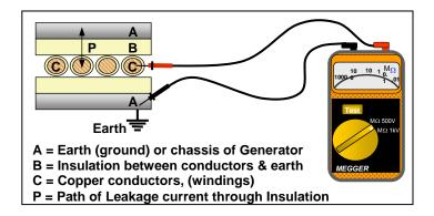
The high voltage causes a current to 'leak' through the insulation system. This current produces an output reading on the Insulation tester ('Megger'), which is measured in Megohms (resistance to earth or ground). A normal value for a low voltage Generator winding should be higher than 1 Megohm to earth.
