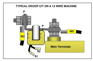
The most important aspect of initial setting up procedure concerns the droop circuit. Most of the troubles allied to poor parallel operation originate from the droop circuit. They are either incorrectly adjusted for the level of voltage droop, or are incorrectly connected, such that a rising voltage characteristic is obtained.
