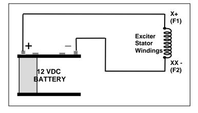
A variable source can be applied to the circuit, as shown: -
