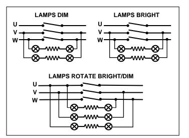
**NOTE:** If the neutral is solidly linked, then only one set of lamp/resistors is required, because the return path is through the neutral link. This, of course, only applies to the lamps dim or lamps bright connection, and not on the three lamp connection. Modern installations prefer to use semi or fully automatic synchronising equipment, which allows breaker closure only when conditions are correct.
