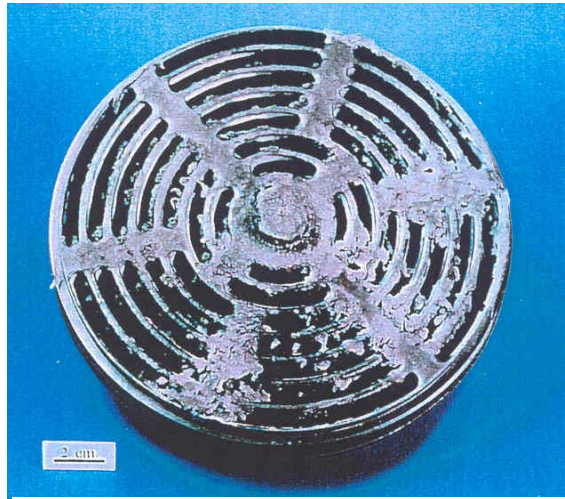
Fig 2 - Plate valve from a PP process compressor - For contaminated gases poppet valves are more suitable
