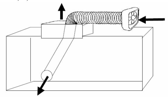
Ventilation should be continuous where possible, because in many confined spaces the hazardous atmosphere will form again when the flow of air is stopped.
