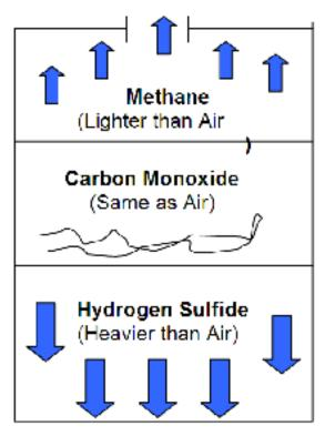
No tank is to be entered until the tank atmosphere has been thoroughly tested with approved and calibrated instruments. Following tests are to confirm that all areas of the tank, bottom in particular, are safe for entry, i.e.:
