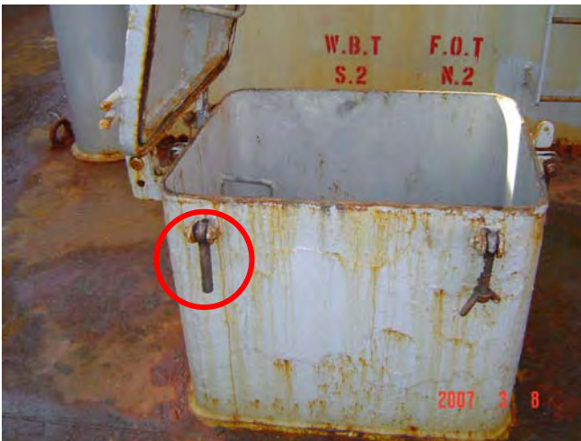
Missing nut of small hatch
