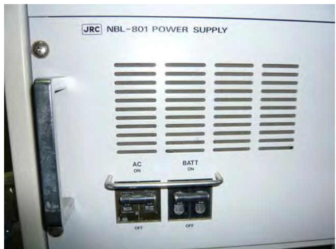
Switch of AC and DC power
