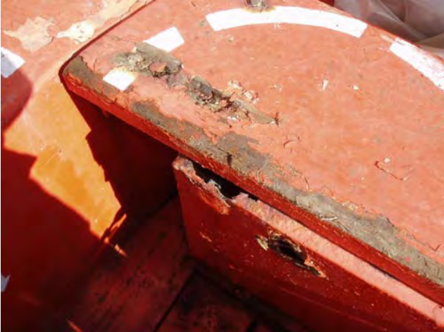
Wasted and broken thwarts
