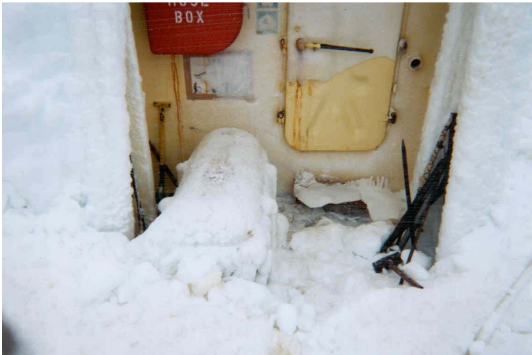
Figures 5.3D – Access to forecabin and forward liferaft severely hampered by presence of ice
