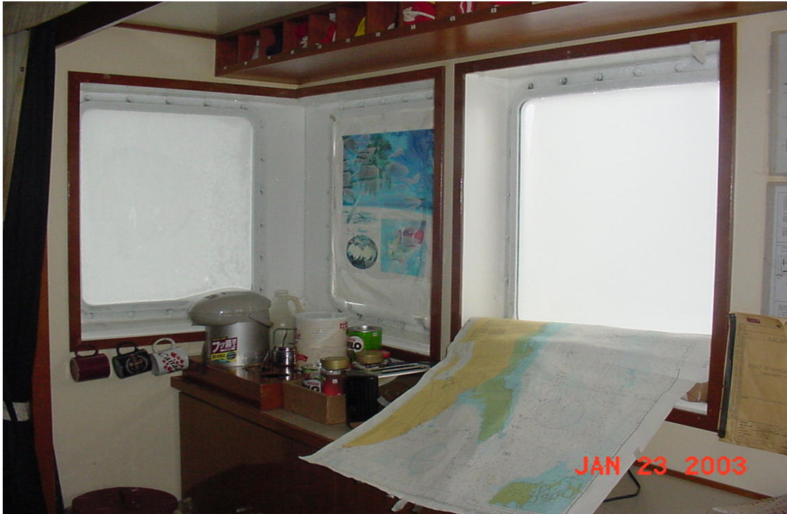
Figure 9.1A – Navigation charts used as insulation, impairing visibility on bridge
