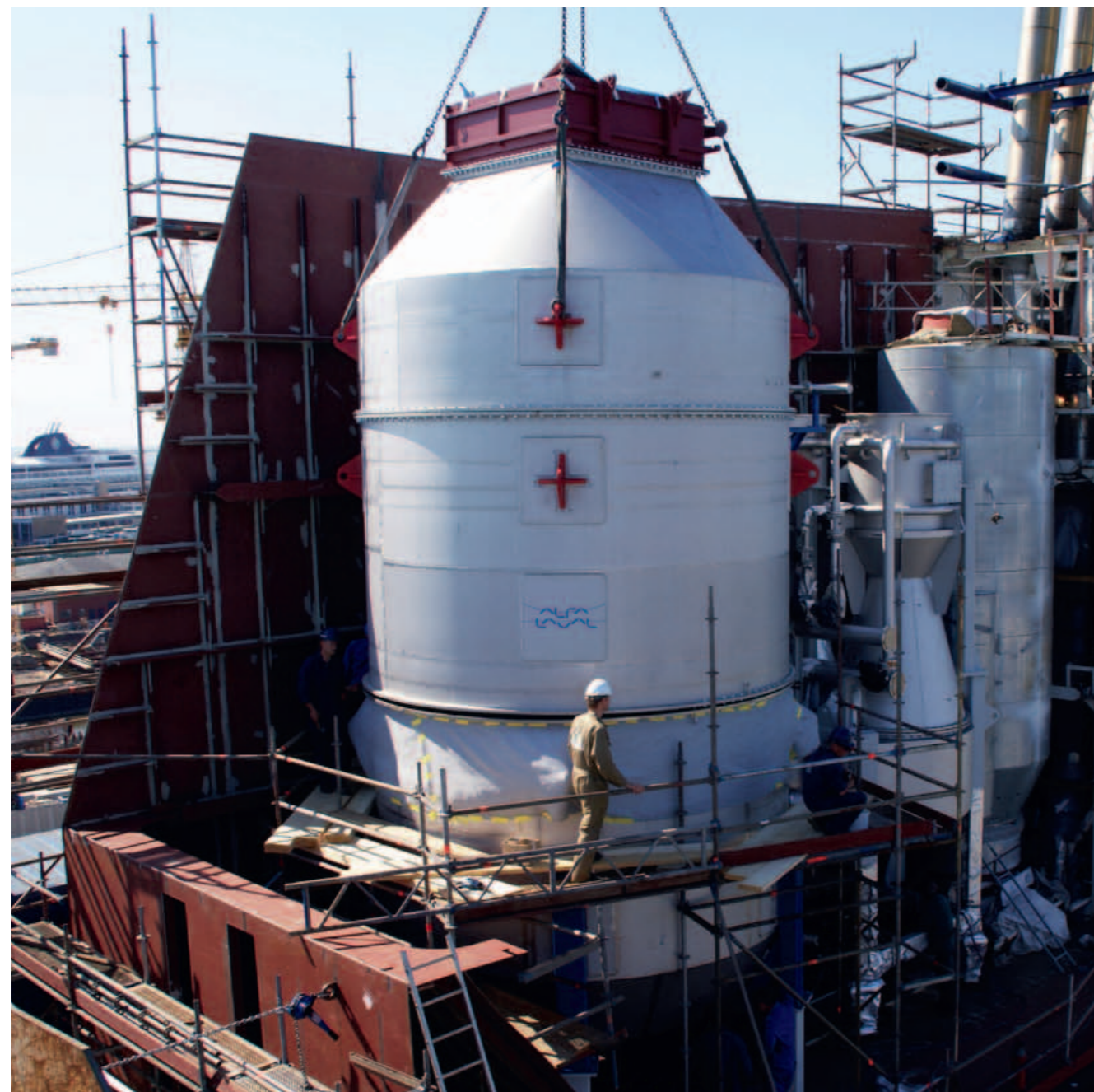
Installing PureSO x on board the Ficaria Seaways.
