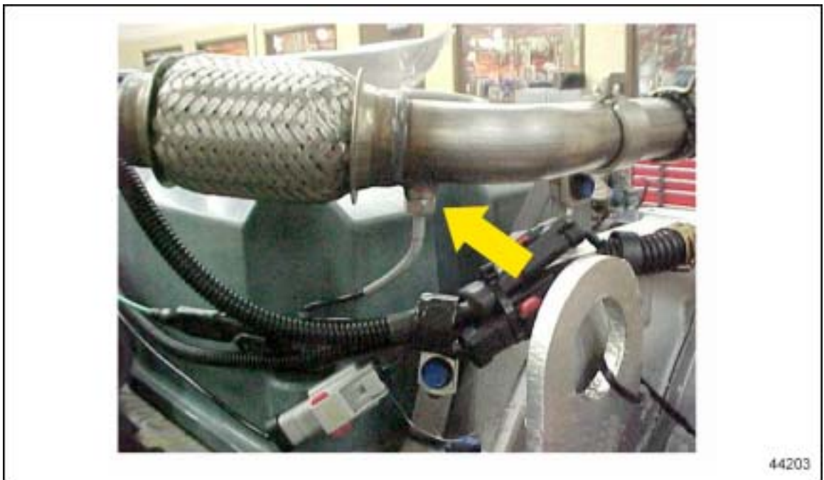
Figure 2-13 EGR Temperature Sensor
