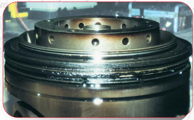
Figure 11: Conventional type lubricant; typical oil scraper ring deposits in a medium speed engine suffering from heavy fuel contamination
