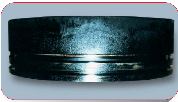
Figure 10: Conventional type lubricant; typical piston deposits in a medium speed engine suffering from heavy fuel contamination
