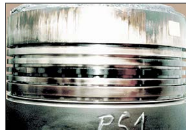
Above: Cleanliness of piston ring area. Below: Cleanliness of piston cooling gallery.
