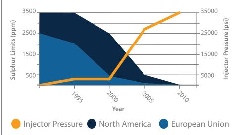
High Pressure Common Rail (HPCR) systems are built to extremely strict tolerances in order to meet emission requirements and reduce consumption. Injector tips are now measured in microns rather than
