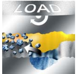
4. Surface fails + created particles
